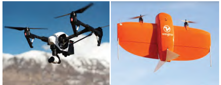
Figure 2. Rotorcraft (left) and fixed-wing (right) drones
