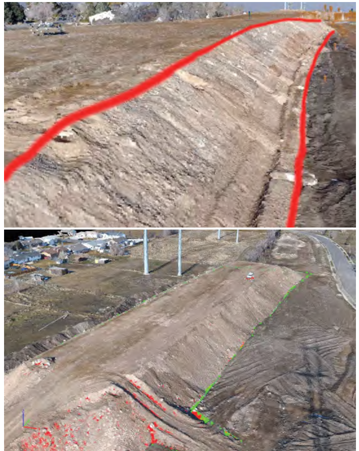
Figure 10. Breakline survey (top) versus point cloud (bottom)
